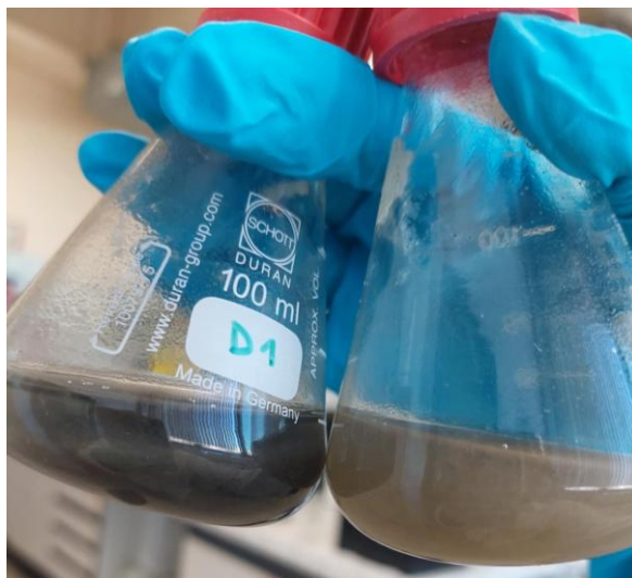
Figure A.3: FeS precipitation in sludge causing the blackish color (left) compared with the same sludge without sulphur dosing (right).
