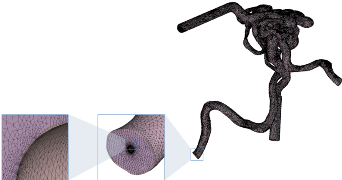
Figure 2.7: The final mesh from Fluent Meshing for the AVM geometry with the implemented catheters. The three boundary layers and mesh refinement around the catheters are apparent on the zoomed-in panels.
