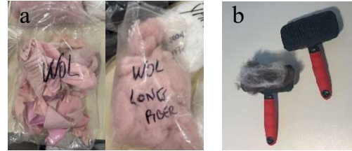
Figure 1: (a): wool in fabric (left) and fiber (right) form; (b) blending the textile and PLA fibers with brushes
