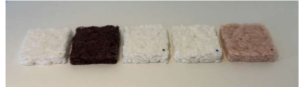
Figure 3: Insulation samples - arranged according to shape retention (ascending from left to right: polyester-acrylic-cotton/polyester blend-cotton-wool)
