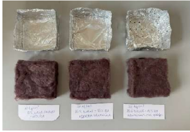
Figure 2: Result 20 kg/m 3 - variation in ratio and contact with hot air
