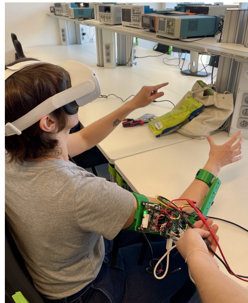
Figure 5.6: User participating in the evaluation wearing the exoskeleton and the HMD
