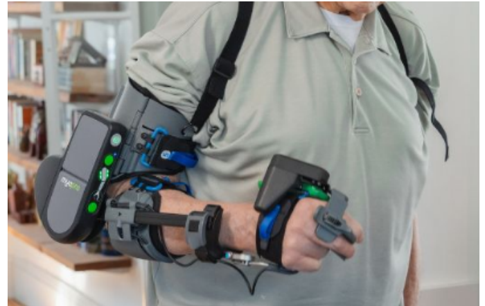
Figure 3.4: Electrically actuated exoskeleton for upper-limb assistance. Adapted from Myomo Inc. [38].
