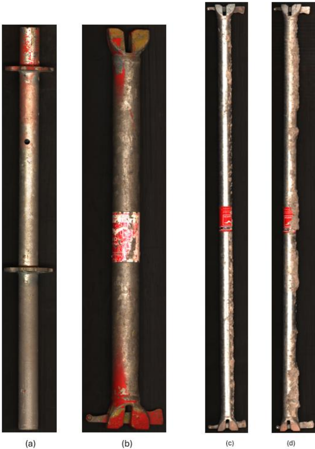
Figure 3-1 presents high-resolution images (to \sim 700 \times 5000 pixels) of captured scaffolding pipes. Pipes (a) and (b) are clean, while (c) and (d) exhibit substantial mortar residue along their length.
