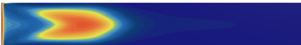
(b) Simulated slug flow.
