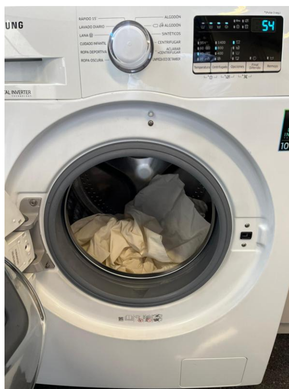
Figure 22: Washing machine set on the wool program (54 min; 40°C; 800 rpm) with the cotton test fabrics inside to simulate domestic laundry conditions.
