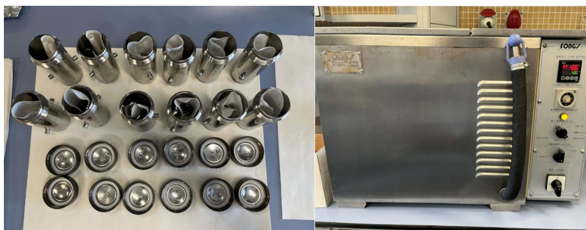
Figure 21: Washing vials containing the test samples, 150 ml of distilled water and 10 steel balls (left), and the Linitest laboratory washing machine (right).
