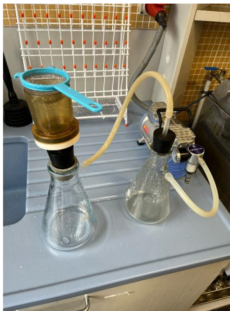
Figure 23: Vacuum-assisted filtering setup.
