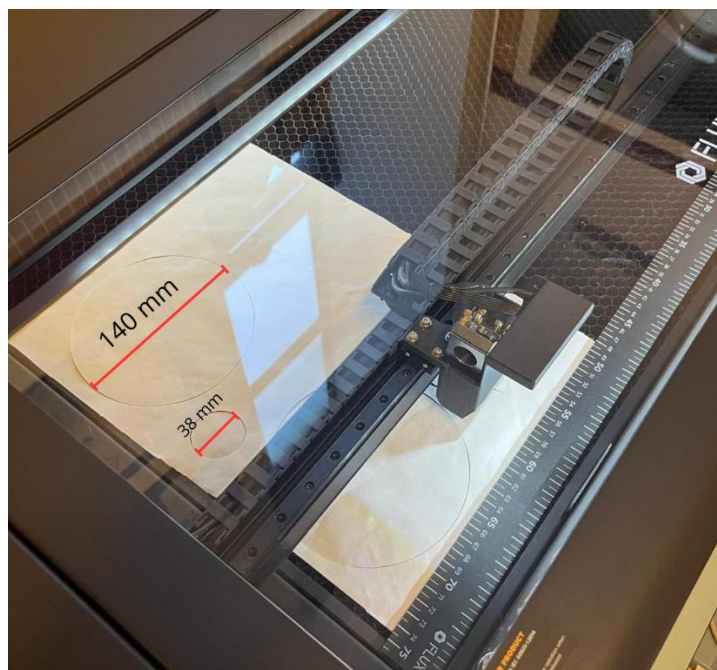
Figure 18: Flux Ador laser cutter preparing the samples for the Linitest with a diameter of 140 mm and 38 mm.
