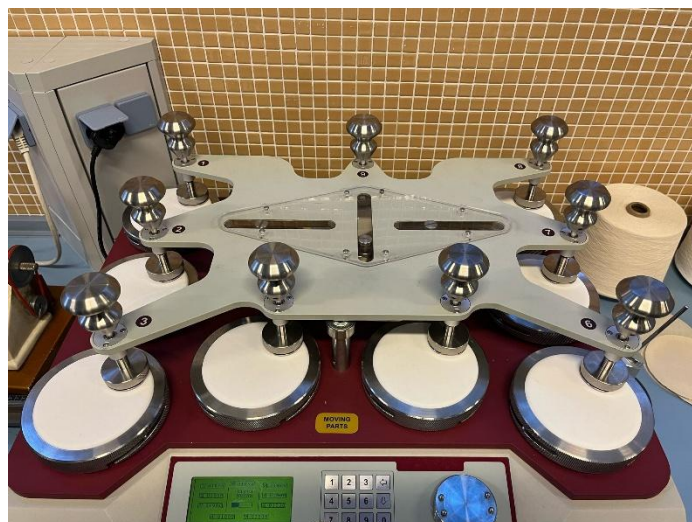
Figure 20: Martindale testing to simulate abrasion.
