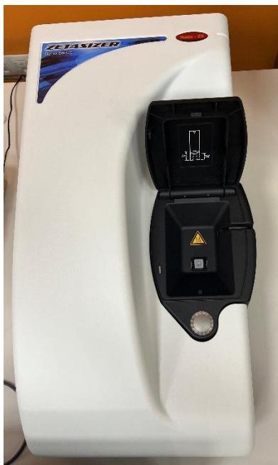
Figure 26: ZETASIZER Nano series DLS device with inserted polystyrene cuvette, containing a filtrate sample.
