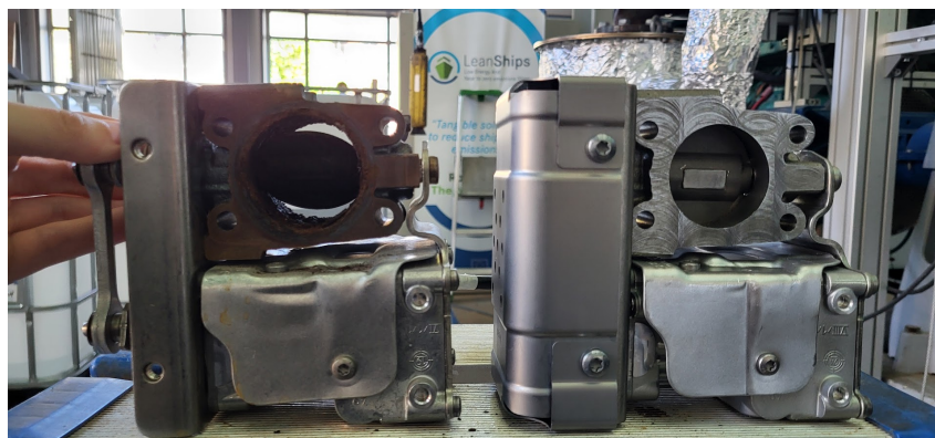
Figure F.3: Corroded EGR Valve (left) and new EGR Valve (right).
