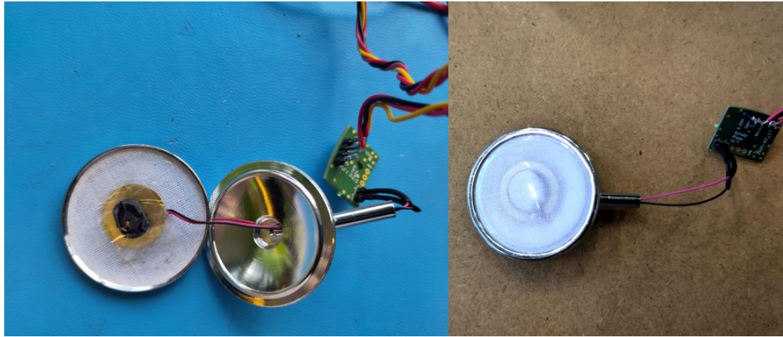
Figure A.7: Piezoelectric transducer mounted behind the diaphragm of a stethoscope chestpiece in combination with a black rubber pen deforming the transducer in response to skin vibrations
