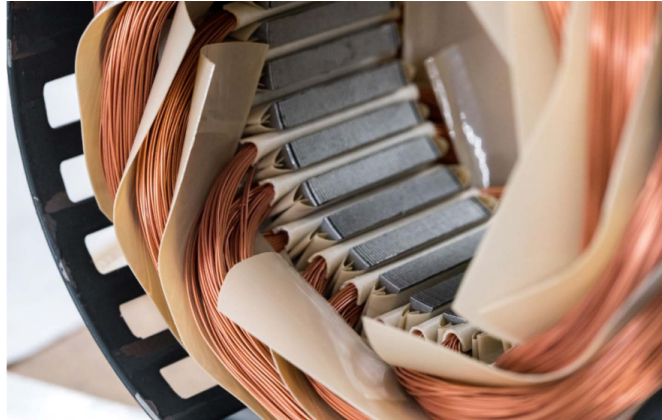
Figure 2.3: Completed stator winding with PEEK material[10]
