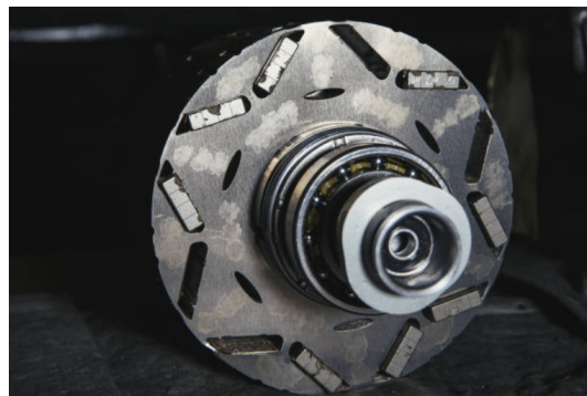
Figure 2.8: Tesla Model 3 rotor configuration [15]
