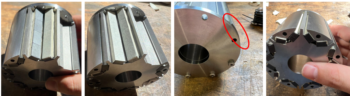
Figure 4.7: Magnet fixation process
