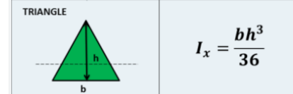
Figure 5.3: Second moment of area for a triangle [21]
