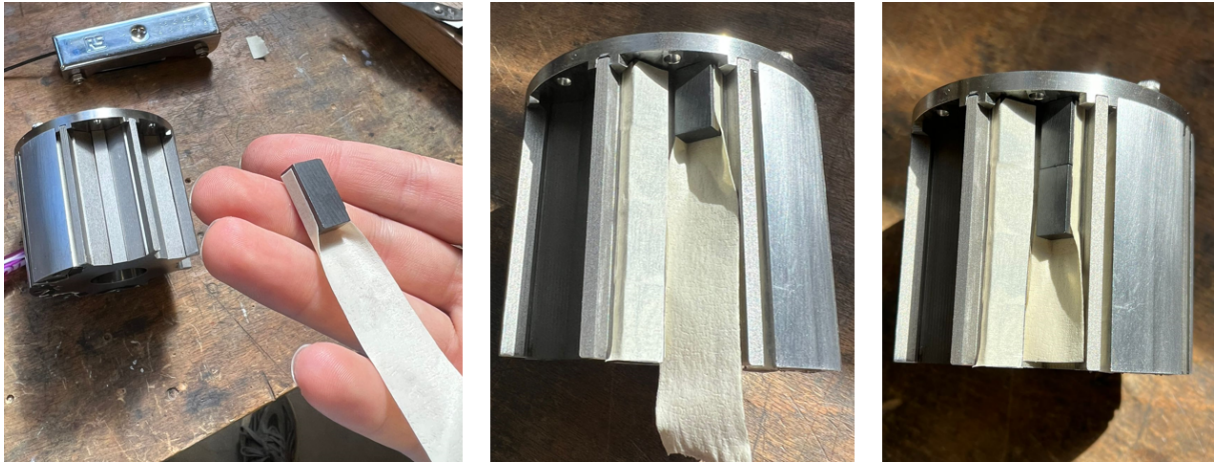
Figure 4.6: Magnet placement process
