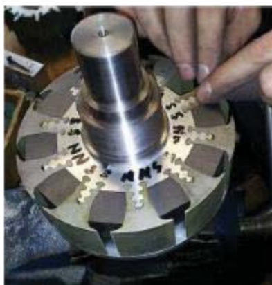
Figure 1.5: Ferrite fir tree rotor[6]
