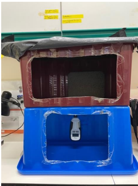
Figure 8. Set-up for PAM (Pulse Amplitude Modulated) fluorescence measurements designed to eliminate ambient light interference. A dark room environment was simulated using two stacked plastic boxes. The PAM probes were inserted through the lower box, while the
