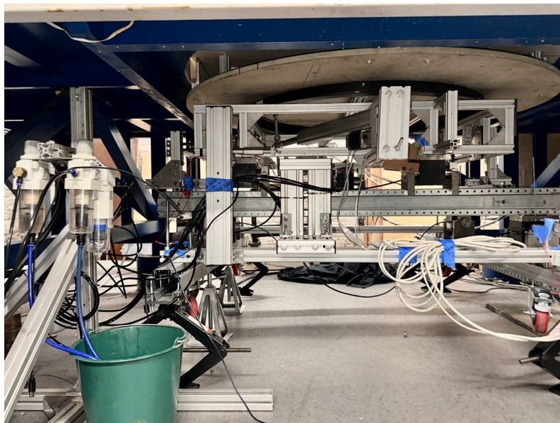
Figure E.2: Balance and turntable seen from below the test-section floor during the first installation under the VUB subsonic tunnel, with the two pneumatic regulators on the left and the signal cabling temporarily routed along the support beam.
