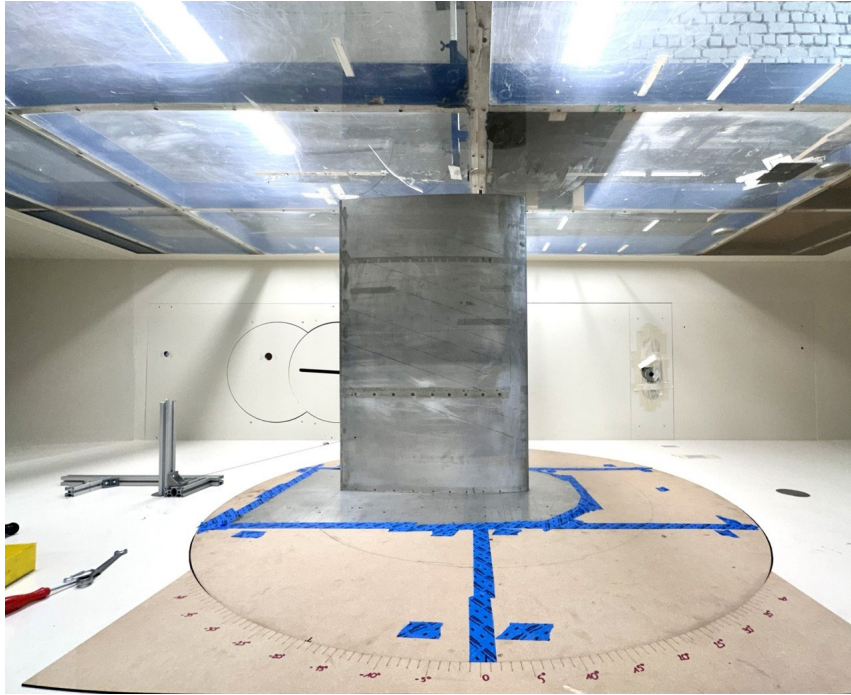
Figure 4.24: NACA 0012 wing mounted vertically on the turntable inside the VUB subsonic tunnel test section.
