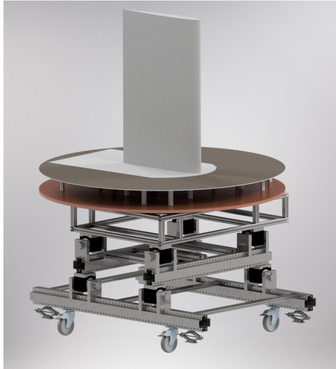
Figure 3.2: CAD render of the balance structure showing the five-layer vertical build-up from the rolling base to the model interface.
