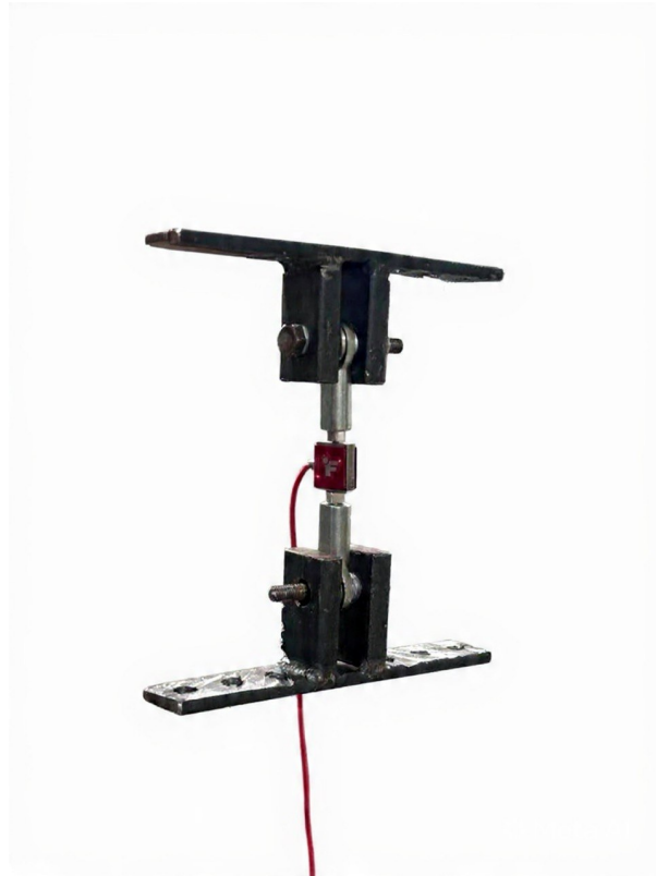
Figure E.5: Load cell clamped between the upper and lower mounting plates of one bushing stage, isolated from the rest of the column. The vertical mounting axis is the cell's sensing direction; the two plates impose the only mechanical path between the moving carriage and the fixed rig.
