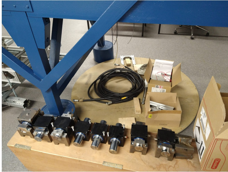
Figure E.1: The BikeValley donation as it arrived at VUB, before reassembly: the eight NewWay porous-graphite air bushings and clamping blocks, the original wooden turntable, the pneumatic hosing, and the steel cross-frame.
