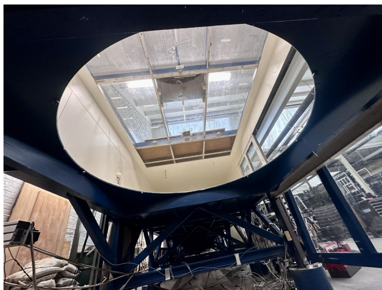
(b) Underside of the test section with the floor panel removed.
