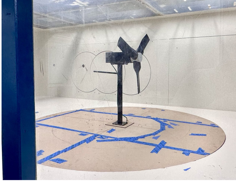
Figure 4.42: Three-bladed scale-model HAWT on motor-driven RPM control inside the VUB tunnel test section.
