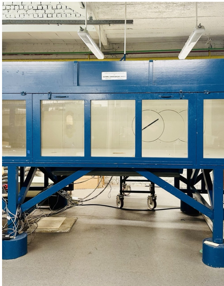
(a) Test section with the original cross-beams in place.
