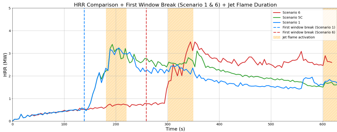
Figure 68: HRR of Scenario 1, 6 and 5C with the window break
