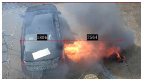
Figure 4: Jet flame release from an EV during a fire event 43
