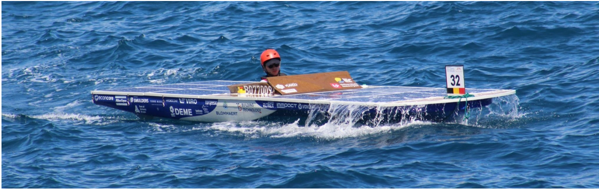
Figure 2.4.: Torpedo MK.II's susceptibility to greenwater and deck-slamming
