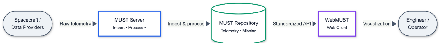
Figure 1: Simplified MUST/WebMUST architecture relevant to the telemetry visualization workflow (adapted from Baumgartner et al., 2005; European Space Agency (ESA), 2024)
