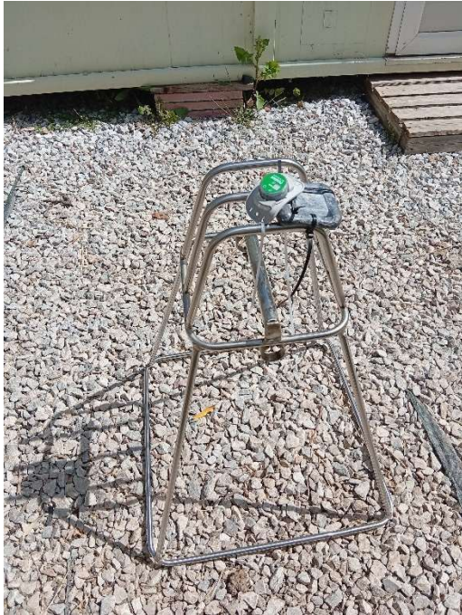
Figure 11: Metal frame with HOBOT logger attached on top used during lionfish surveys to measure water temperature and light intensity.
