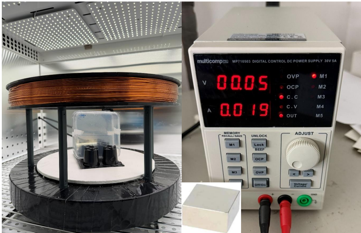
Figure 4 A pair of identical circular Helmholtz coils (diameter 40 cm, left image) arranged coaxially and separated by a distance equal to the radius (20 cm), generating a uniform magnetic field in the central region. Each coil consists of 200 loops of copper wire and is supplied with a controlled electric current. Experimental samples are positioned centrally between the coils, where the magnetic field is most homogeneous. The direction of the generated magnetic field can be adjusted to either enhance the ambient GMF or to counteract its vertical component, thereby creating weak magnetic field conditions. The power supply which was used (right), set to a Voltage and current to cancel out the vertical component of Earth's magnetic field. The permanent magnet type used alongside the coils is displayed in the lower centre.
