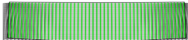
Figure 3.26: Grid distortion of the 2D scanning multispectral imager with F/4.5 for the on-axis field. Green crosses inside the black contour represent the real grid points, and the black lines represent the vectors connecting the real with the ideal grid points. The grid size is 50 \times 50 . Field width is 48^\circ . Aspect ratio is 0.208.
