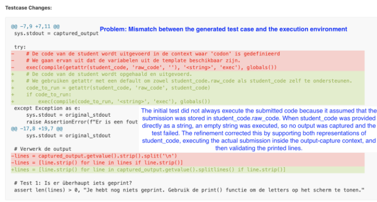
FIGURE I.2: Solved: Source was a mismatch between test generation and the execution environment
