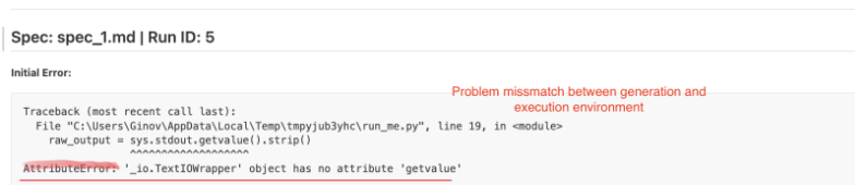
FIGURE I.5: The solution code was not executed
