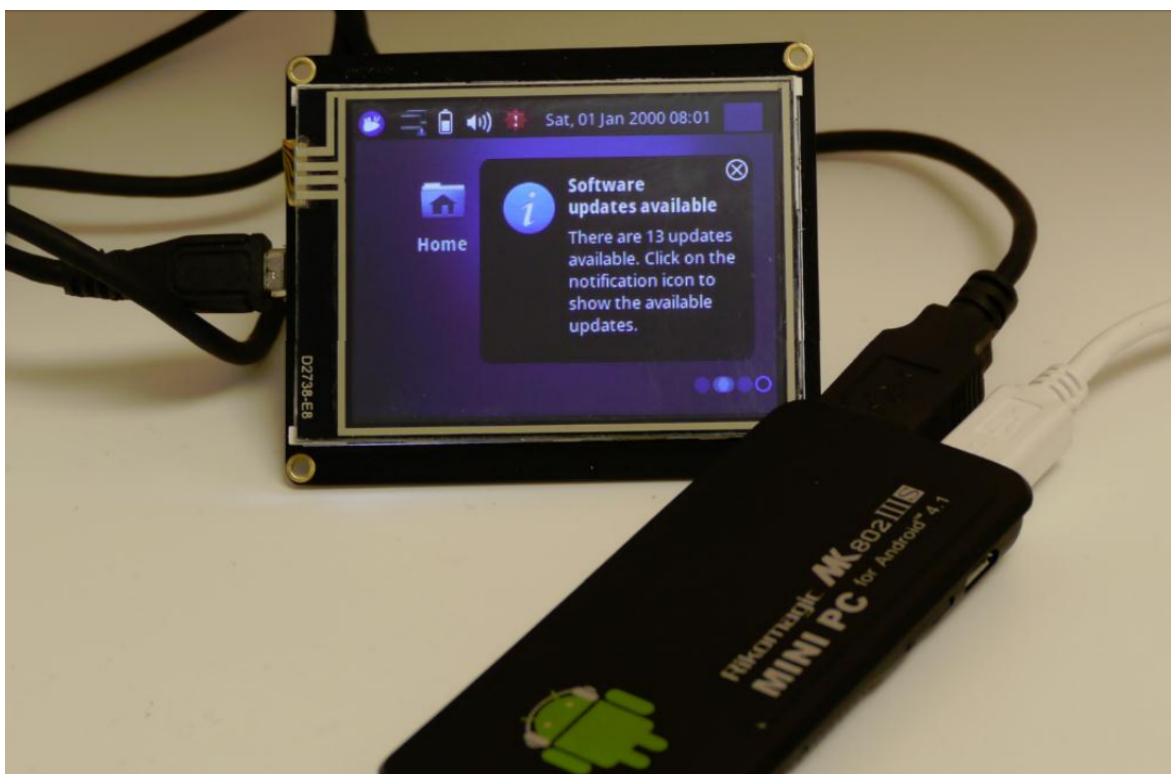
Figure 10.2: A USB display used as a primary display on a Mini PC, showing the Ubuntu desktop. Image obtained from RoboPeak (2013).
