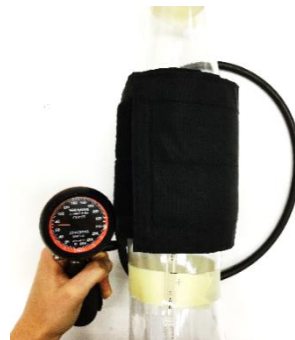
Figure 4 The calibration of the plastic leg with the help of a sphygmomanometer.
