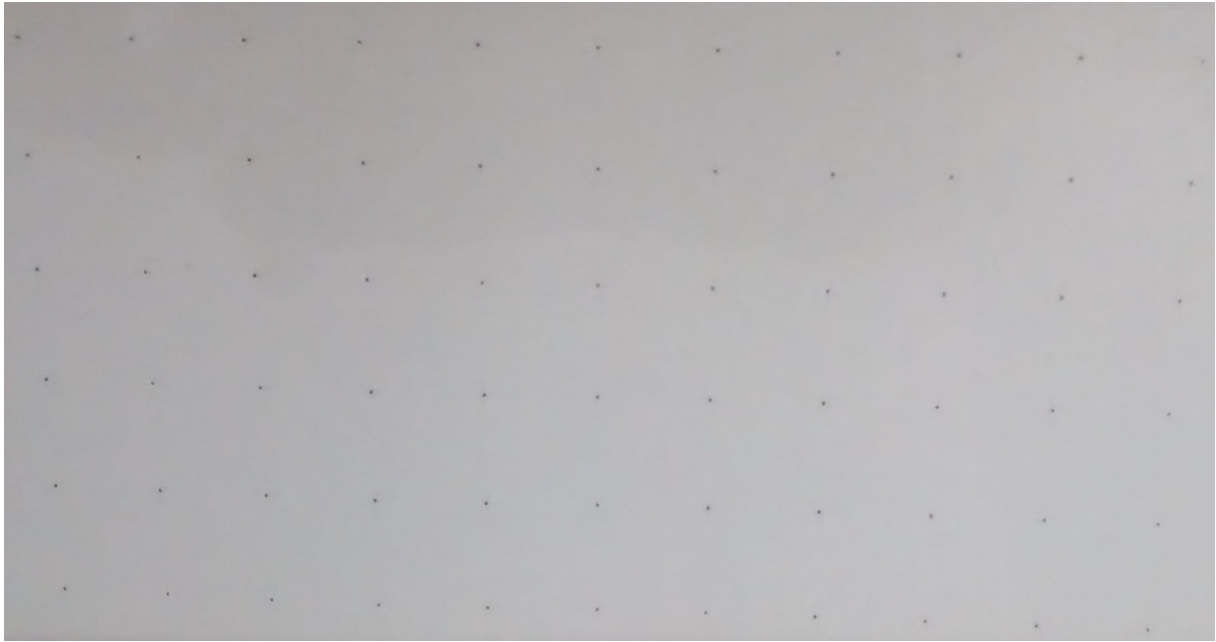
Figure 5.9: Adopted feature pattern during this thesis, consisting of regularly spaced dots with a diameter of 0.1 mm and a spacing of 10 mm.
