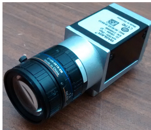
Figure 6.2: Area scan Basler ace GigE camera, equipped with a Basler lens with focal length of 8 mm
