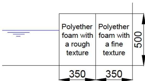
Figure 3-13: Side view of the vertical wall of polyether foam
