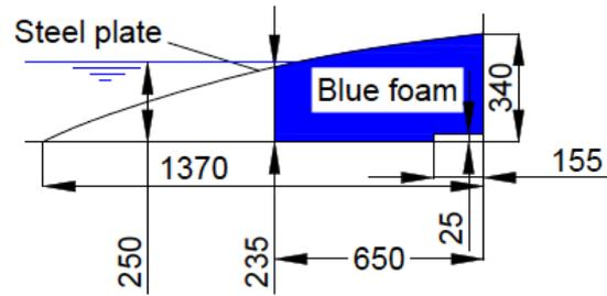
Figure 3-9: Side view of the parabola with blue foam for a water level of 25 cm
