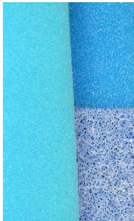
Figure 4-19: Different types of foam used as an absorbing material in the test program
