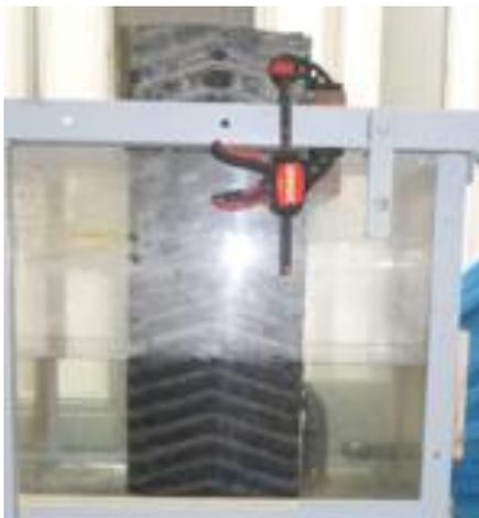
Figure 7 Hexablock installed in the wave flume
