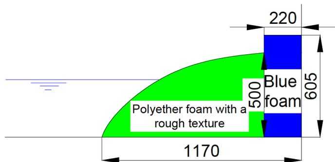
Figure 3-15: Side view of the parabola of polyether foam
