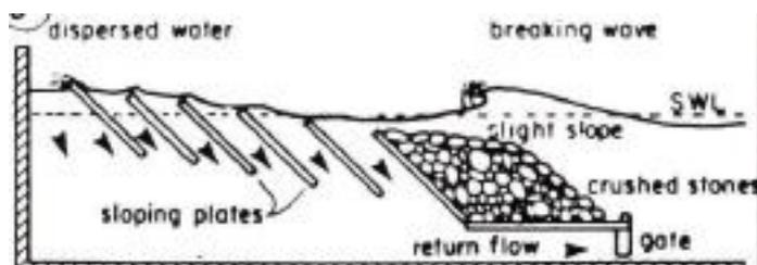
Figure 2-13: Submerged slope [15]
