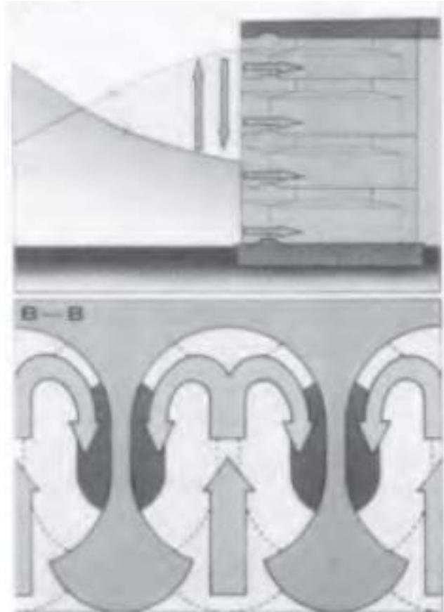
Figure 2-28: Principle sketch of the Igloo wave absorber - the lower part is showing the cylindrical chambers inside the blocks [16]
