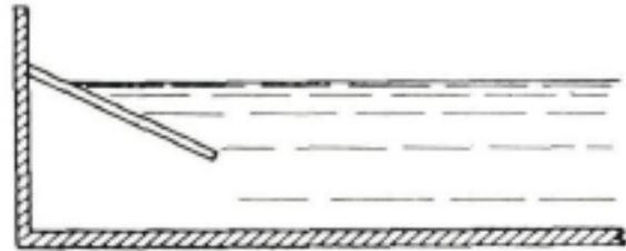
Figure 2-5: Sloping beach that doesn't reach the bottom [15]
