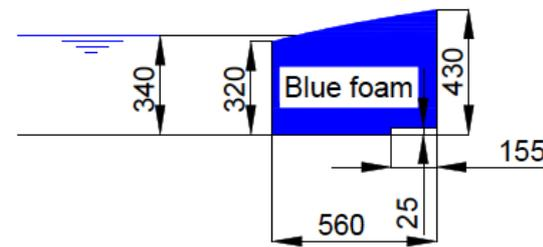
Figure 4-6: Side view of the blue foam absorber for a water level of 34 cm
