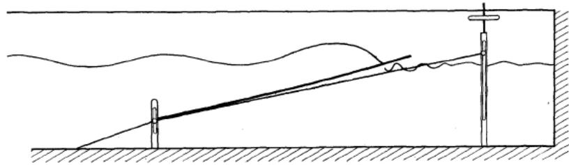
Figure 2-11: Marcou wave absorber between two wave attacks [12]
