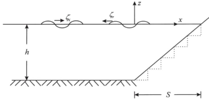
Figure 2-3: Standard sloping beach as a N-step staircase [24]
