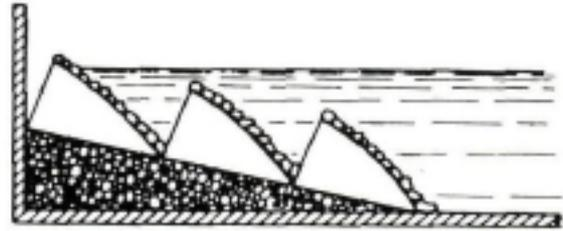
Figure 2-18: Combination of a straight and a parabolic slope [15]
