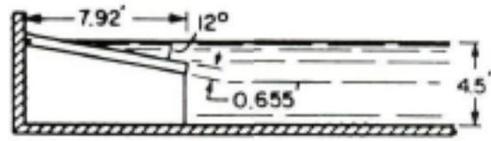
Figure 2-9: Slope with a front wall [15]
