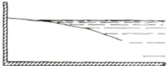
Figure 2-8: Broken slope that doesn't reach the bottom [15]
