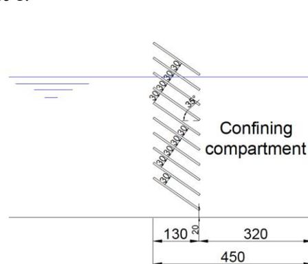
Figure 1 Side view of the Superposed and Inclined Planes Wave Absorber
