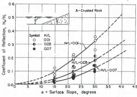
Figure 2-2: Reflection coefficient in function of slope-angle for crushed rock [17]
