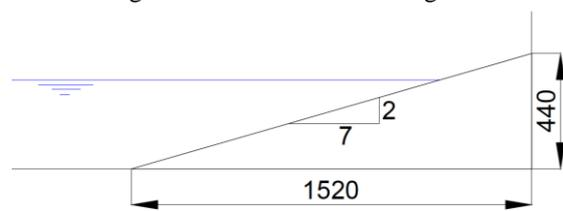
Figure 4 Side view of both sloping beaches
