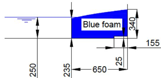
Figure 4-5: Side view of the blue foam absorber for a water level of 25 cm
