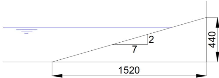
Figure 3-2: Side view of the two sloping beaches
