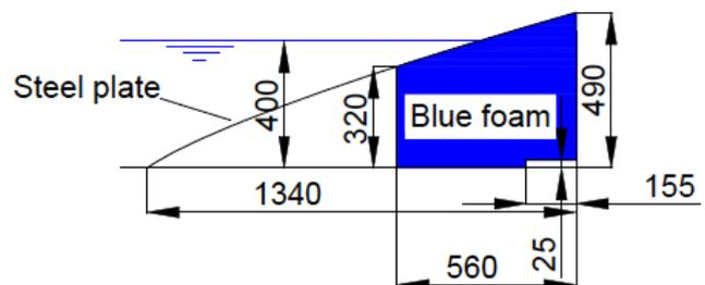
Figure 3-7: Side view of the parabola with blue foam for a water level of 40 cm
