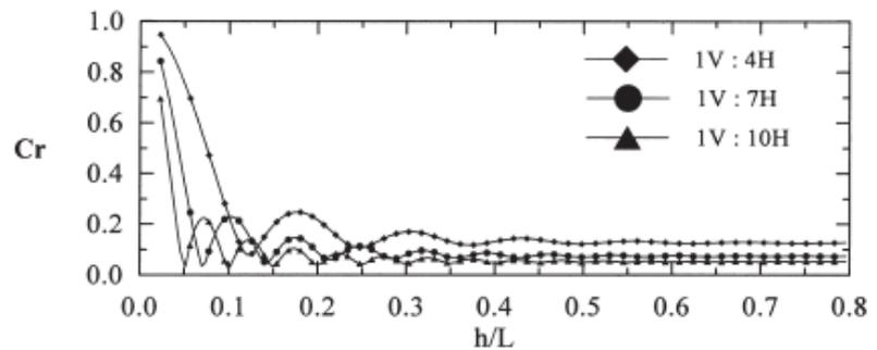
Figure 2-4: Reflection coefficients for different slopes [24]
