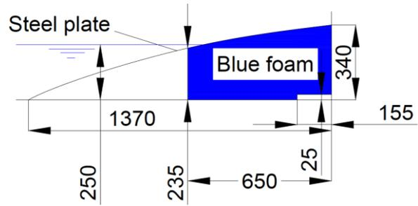
Figure 3 Side view of the porous parabola with blue foam
