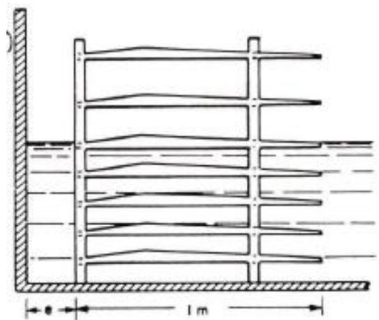
Figure 2-27: Superposed planes wave absorber [15]
