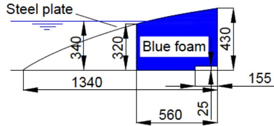
Figure 3-8: Side view of the parabola with blue foam for a water level of 34 cm
