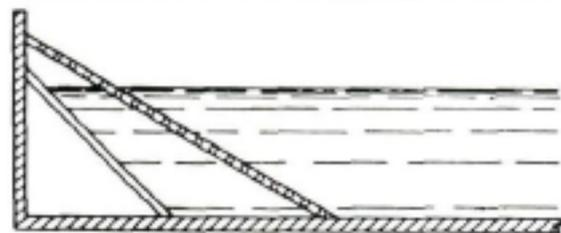
Figure 2-6: Sloping beach with a mesh in front [15]
