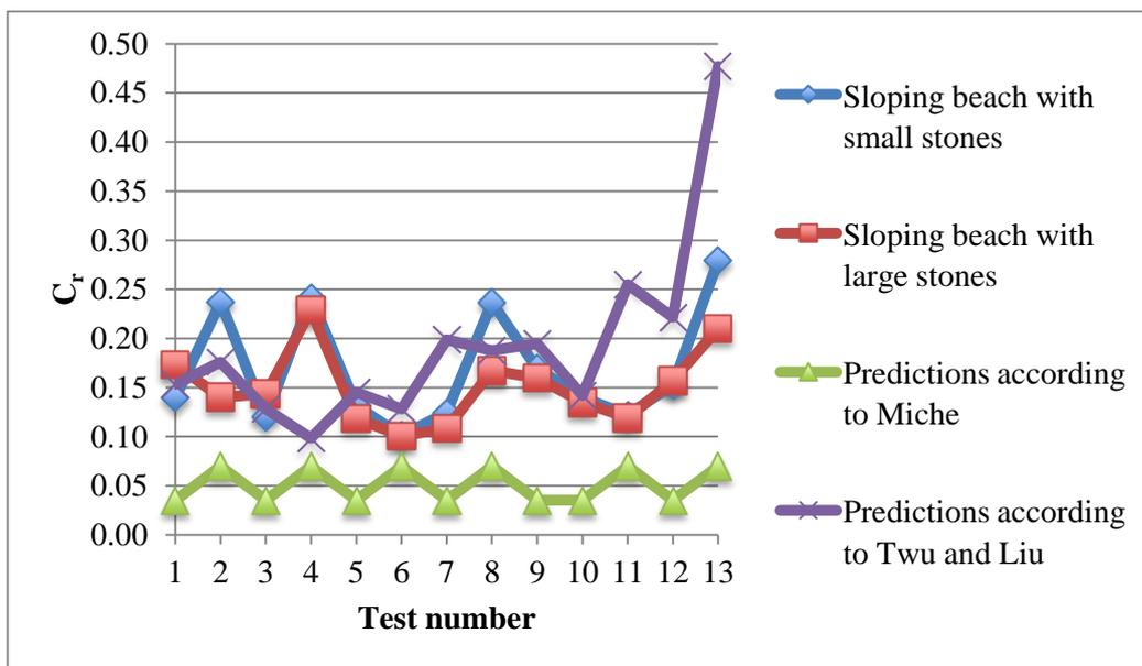
Figure 4-18: Comparison between measured and predicted reflection coefficients
