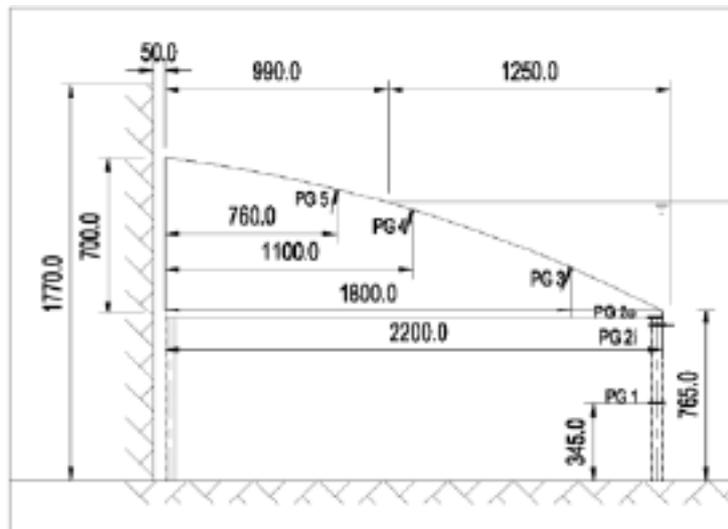
Figure 2-17: Parabolic slope with a front plate [19]
