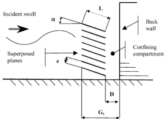
Figure 2-25: Superposed and Inclined Planes Wave Absorber [9]
