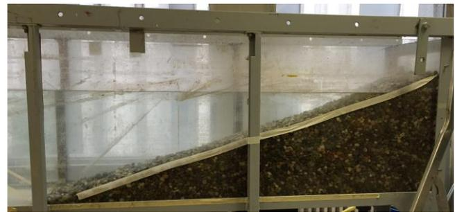
Figure 3-3: Picture of the sloping beach with small stones
