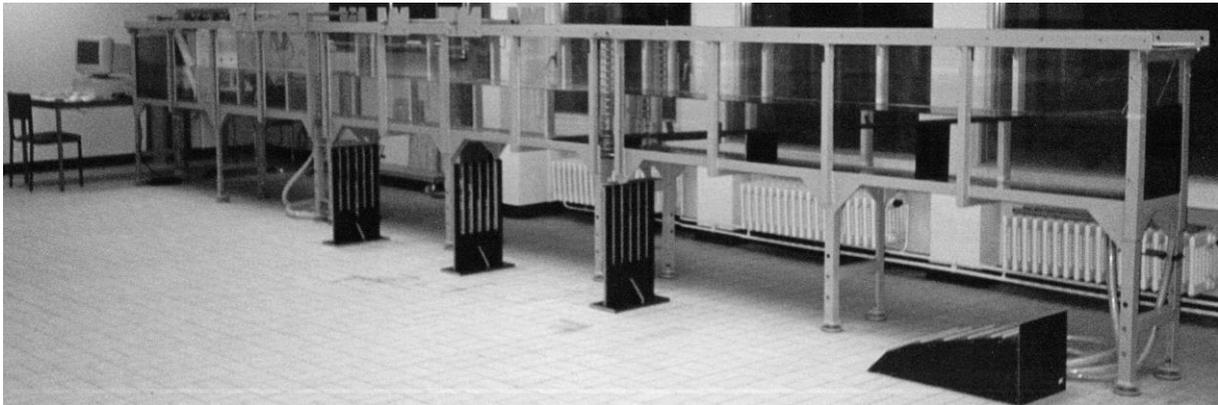
Figure 3-1: The small wave flume of the department of Civil Engineering [3]
