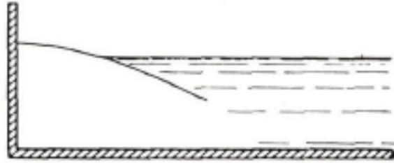
Figure 2-16: Parabolic slope that doesn't reach the bottom [15]
