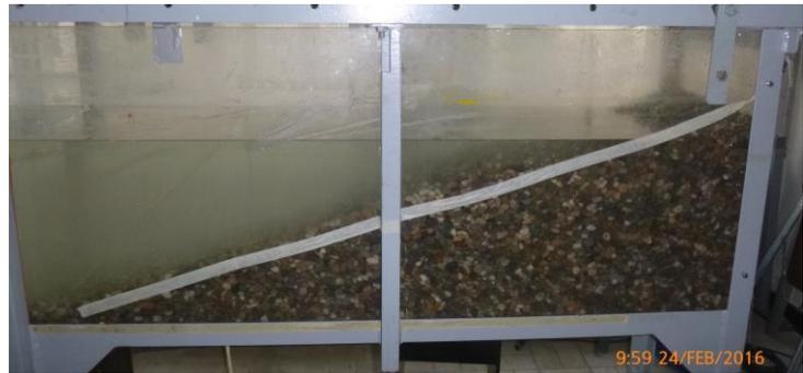
Figure 3-20: S-profile observed in the profile of the sloping beach with small stones
