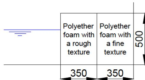
Figure 5 Side view of the vertical wall of polyether foam
