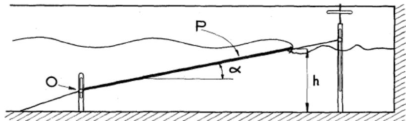
Figure 2-10: Marcou wave absorber during wave attack [12]
