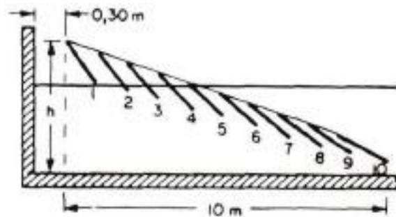
Figure 2-14: Perforated slope [15]
