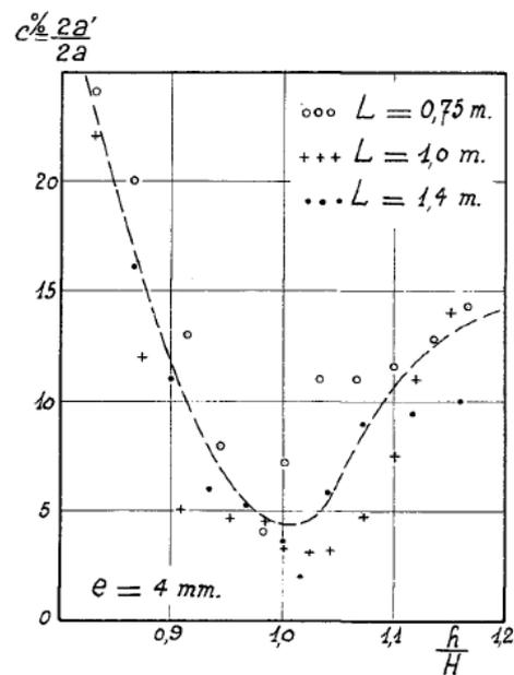
Figure 2-12: Reflection coefficient in function of  $h/H$  for a plate-thickness of 4 mm [12]
