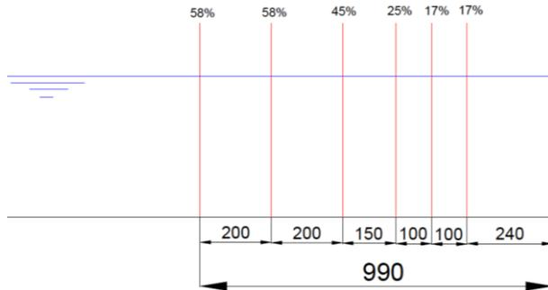
Figure 2 Side view of the vertical mesh absorber. The porosities of the different plates used in the vertical mesh are mentioned above each plate. Dimensions are in millimetres.
