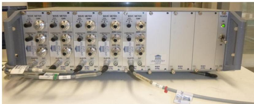
Figure 3-22: Measuring device for wave gauges
