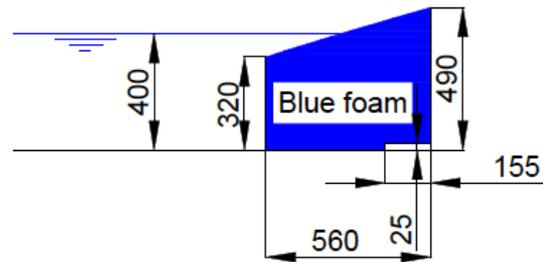
Figure 4-7: Side view of the blue foam absorber for a water level of 40 cm
