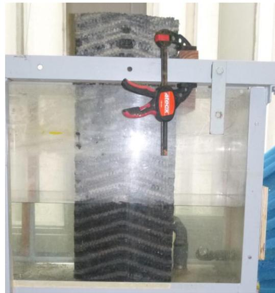
Figure 3-18: Picture of a hexablock installed in the flume
