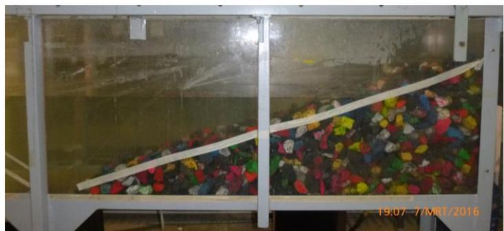
Figure 3-4: Picture of the sloping beach with large stones
