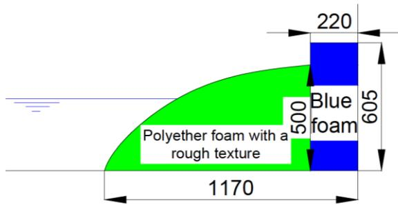
Figure 6 Side view of the parabola made out of polyether foam
