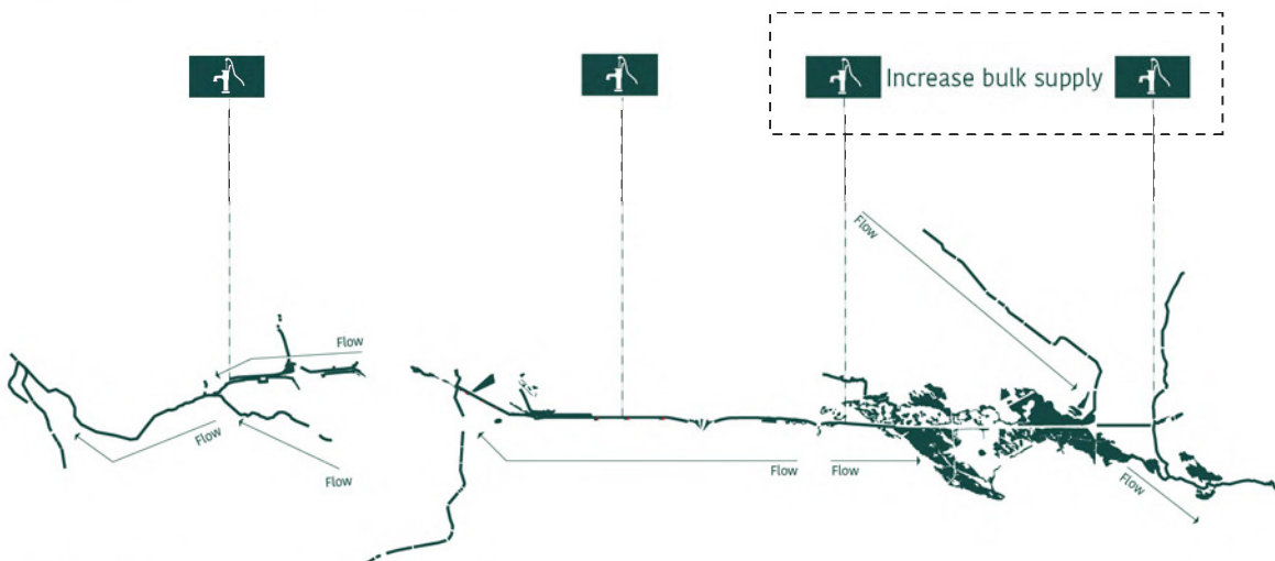
Waterline with aquifer pumps and constructed wetlands
