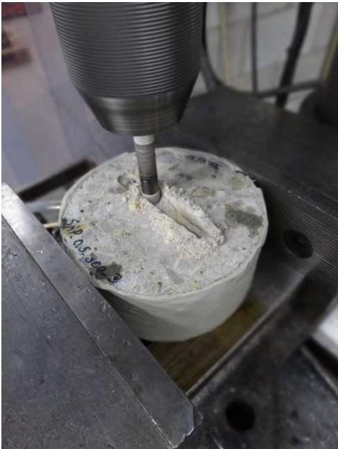
Figure 29: Grinding using diamond drill head mounted on column drill
