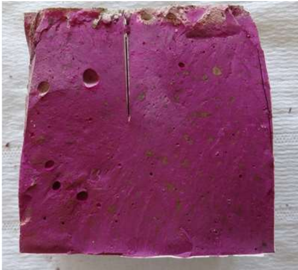
Figure 67: Limited carbonation around artificial crack in cement paste; 12 weeks of exposure
