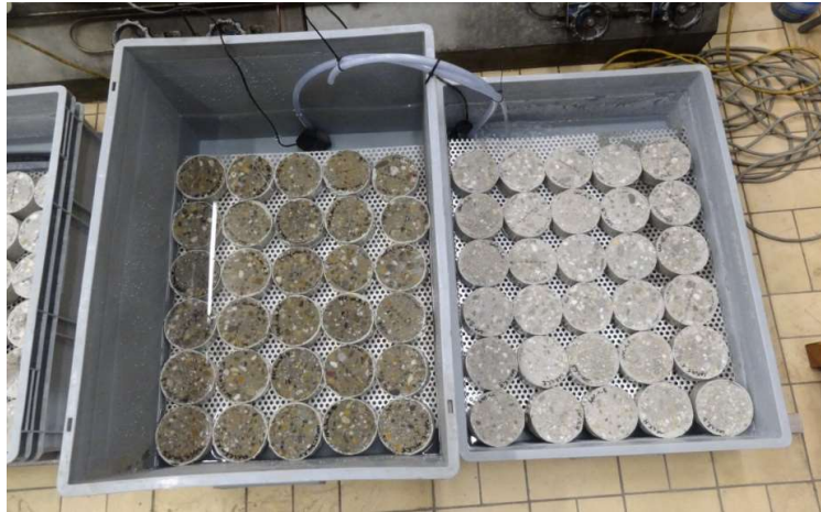
Figure 24: Test setup for wet-dry cycles
