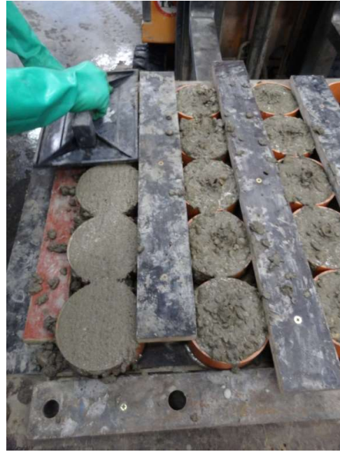
Figure 14: Flattening of the sample surface
