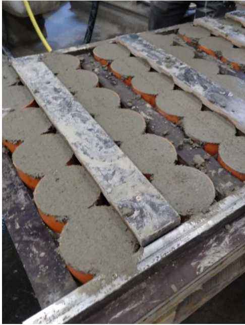
Figure 13: PVC moulds clamped on wooden base
