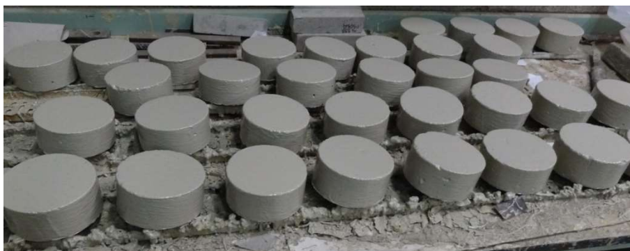
Figure 15: Coating of the non-exposed sides with a two-component epoxy
