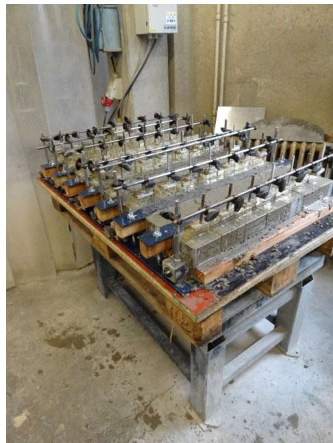
Figure 12: Compaction with vibrating table
