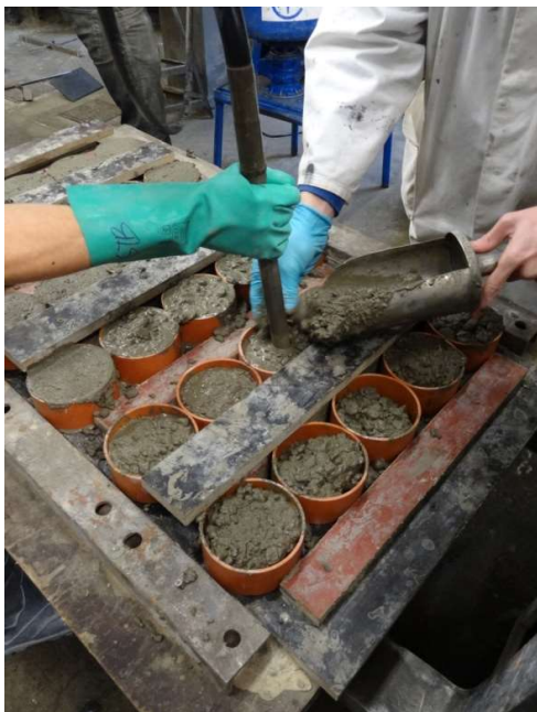
Figure 11: Compaction with poker-vibrator
