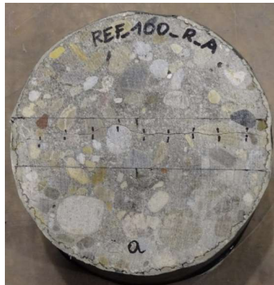
Figure 19: Example of a realistic crack of 100 \mu\text{m} obtained with the crack-width controlled splitting test
