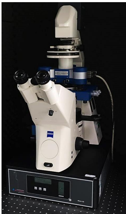
Figure 36. Contact-mode AFM set up.
