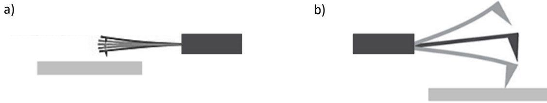
Figure 27. a) ‘Non-contact mode’ AFM: image acquisition occurs without contacting the surface of the sample. b) ‘Tapping-mode’ AFM: the oscillating tip-cantilever system is brought in intermittent contact with the surface and is then raster scanned across the sample. The oscillation amplitude applied to the vibrating system is significantly larger than in ‘non-contact mode’ AFM. [52]
