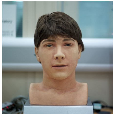
(d) Jules, Hanson Robotics, (Jaeckel et al., 2008), has a skin made of Frubber.
