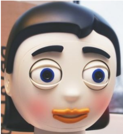
(a) Flobi, which has rigid and flexible facial components. (Lütkebohle et al., 2010)
