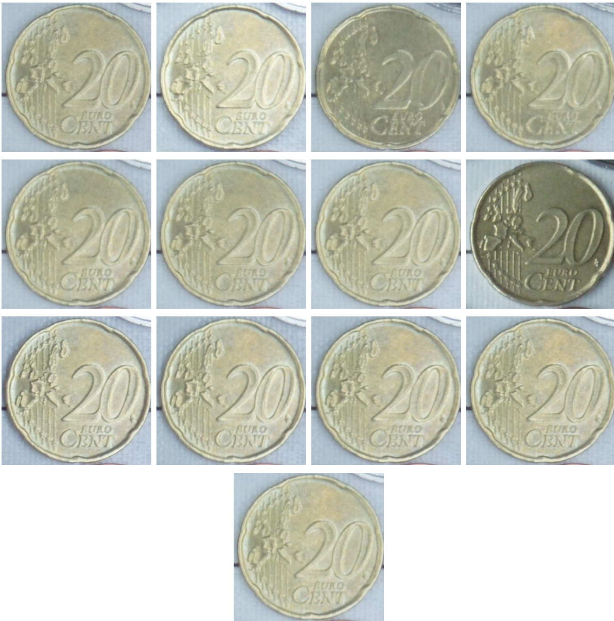
Figure 6.10: Pixel codification real-world results (coin): simulating 4096 single light source images with 13 images lit by coded patterns.
