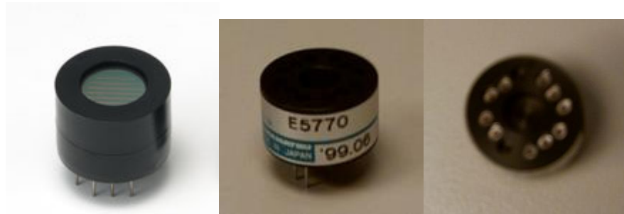
Figure 120: Left: PMT R7400U-01 [HA74]; Right: pictures taken from the active socket.
