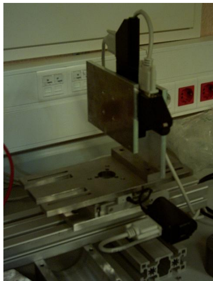
Figure 33: Mounting plate of the detector box, driven by three independent electro motors.
