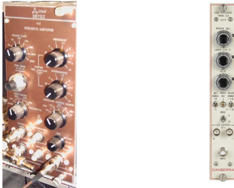
Figure 122: Left: picture of the ORTEC450 Right: single channel analyzer 2037 A [CA09].
