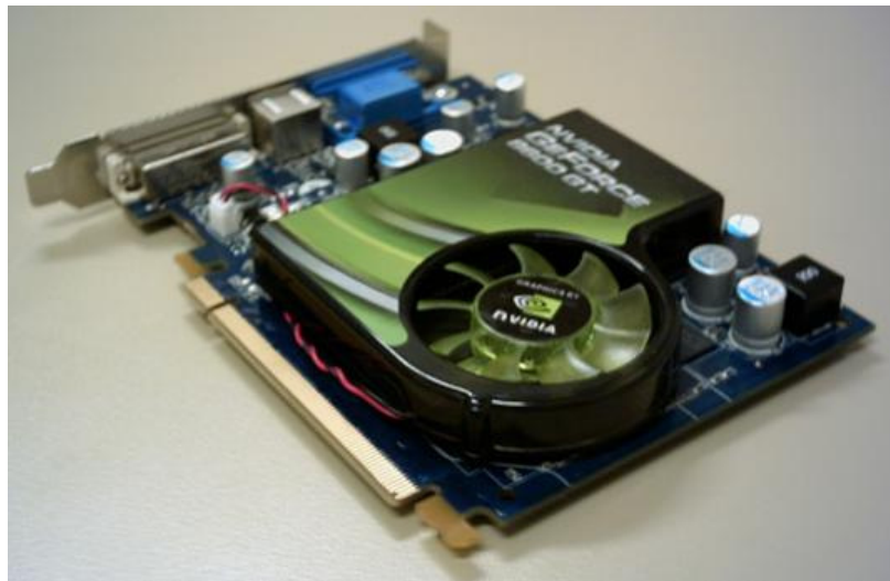
Figure 117: The used GeForce 8600 GT.
