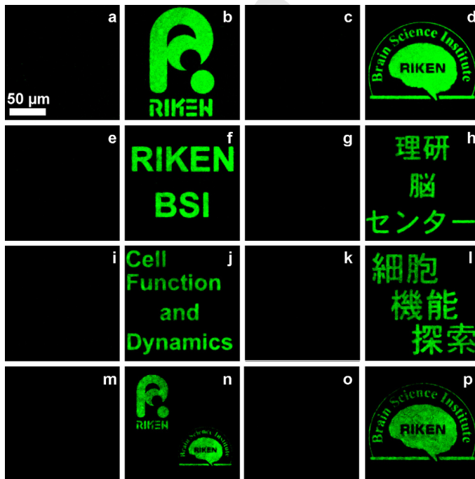
Fig. 2. 2D reversible data storage using Dronpa. The photochromic fluorescent protein Dronpa was cross-linked on a surface coated with poly-L-lysine. The whole field of view of this surface was then illuminated 488-nm laser light (5.5 kW/cm 2 , pixel dwell time 10 µs, five scans) to switch the protein to its non-fluorescent state (a, c, e, g, i, k, m, o) and by a weak 405-nm laser light (332 W/cm 2 , pixel dwell time 10 µs, two scans) to switch the protein back to its fluorescent state, drawing defined patterns (b, d, f, h, j, l, n, p). Using this method, the logos of the RIKEN, Brain Science Institute and laboratory for cell function and dynamics, both in English and Japanese were sequentially drawn and erased on the very same surface. The images were obtained by scanning the surface with 488-nm light (113 W/cm 2 ). The contrast between bright and dark molecules is excellent although after several cycles, a certain photofatigue of the protein can be noticed as one can see by comparing images d and p.
