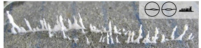
Figure 4 Formation of stalactites at the bottom of the specimens after the permeability test.
