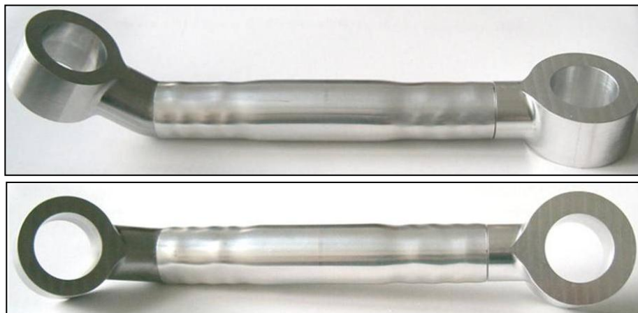
Figure 1.3: Example of an application of the electromagnetic pulse crimping [3].
