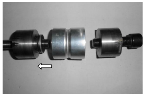
Figure 4.8: The first cylinder can now be pushed out of the deformed tube.
