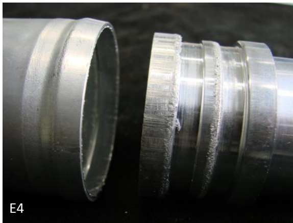
Figure 5.22: Tensile test sample of test series E (45.4 kN).
