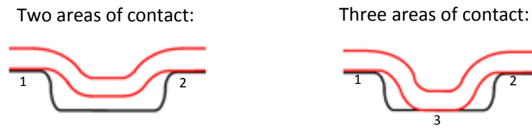
Figure 4.12: The leakproofness of the crimp joint is improved when the tube touches the bottom of the groove.
