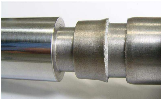
Figure 3.8: Failed axial crimp joint (sample 6).
