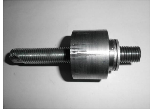
Figure 4.2: First (left) cylinder and positioning rings placed on the threaded rod.
