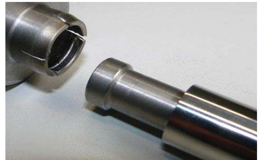
Figure 3.9: Failed axial crimp joint (sample 15).
