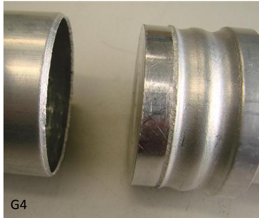
Figure 5.26: Tensile test sample of test series G (37.9 kN).
