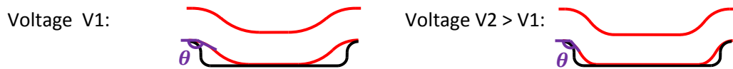
Figure 6.22: A larger voltage creates a stronger interference fit and a stronger mechanical interlock.
