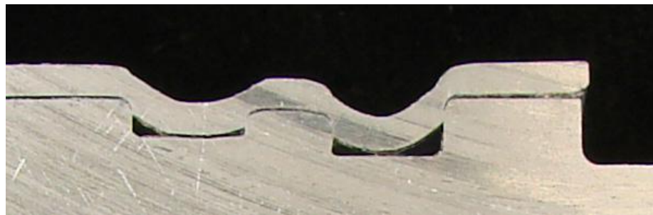
Figure 1.1: Electromagnetic crimp joints obtain their strength from the combination of an interference and a form fit.
