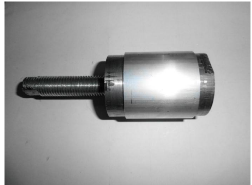
Figure 4.4: Aluminum tube is positioned over the cylinder system.
