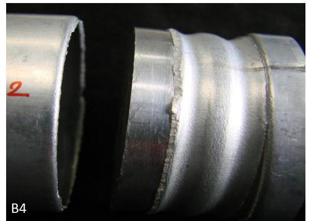
Figure 5.11: Tensile test sample of test series B (23.2 kN).
