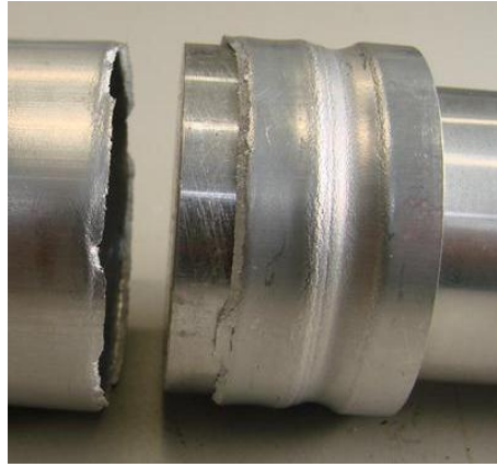
Figure 5.29: Tensile test sample of test series H (53.8 kN).
