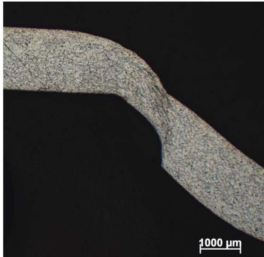
Figure 4.29: Shearing at the groove edge.
