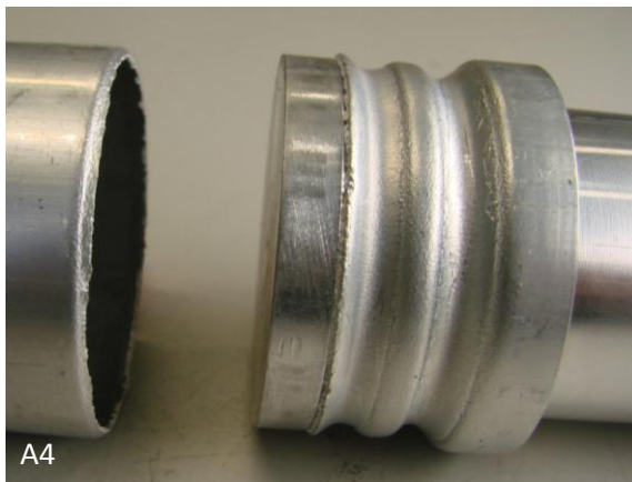
Figure 5.10: Tensile test sample of test series A (39.9 kN).
