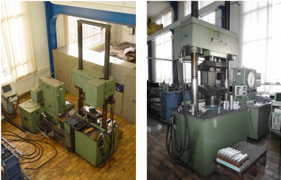
Figure 3.4: Amstler universal testing machine in Laboratory Soete [35].
