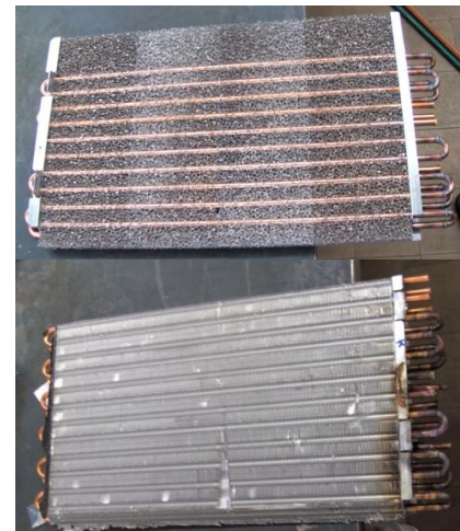
Fig. 1. Two identical heat exchangers: metal foam (at the top), louvered fins (below)
