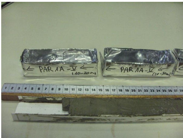
Fig. 11: Aluminum boxes and U-channel with sediment ready for sub-sampling
