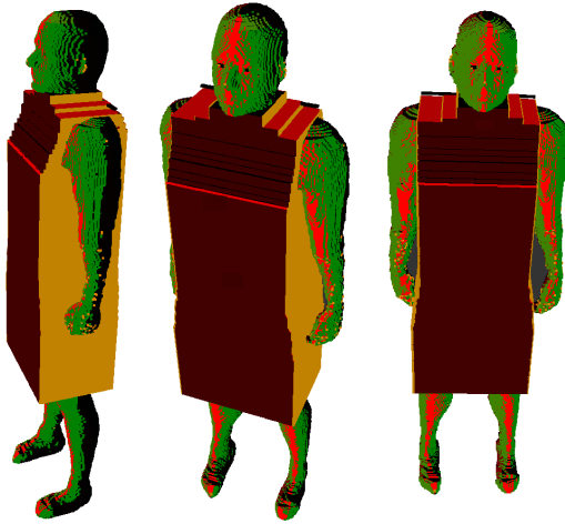
Fig. 2. Three-dimensional image of the optimized and validated MAX phantom extended with lead apron and a thyroid protector.
