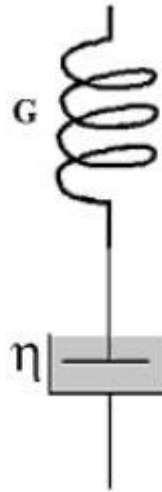
Figure 1.5: A spring and a dashpot element joined in series, a model of the Maxwellian viscoelastic liquid (Malkin, Malkin et al. 2006)
