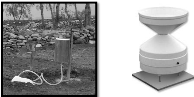
Figure 3.7 Left - Non automatic rain gauge for measuring daily rainfall depths. Right – data logging tipping bucket rain gauge for rainfall intensities
