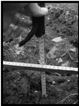
Figure 3.12 Example of the measurement of soil surface roughness
