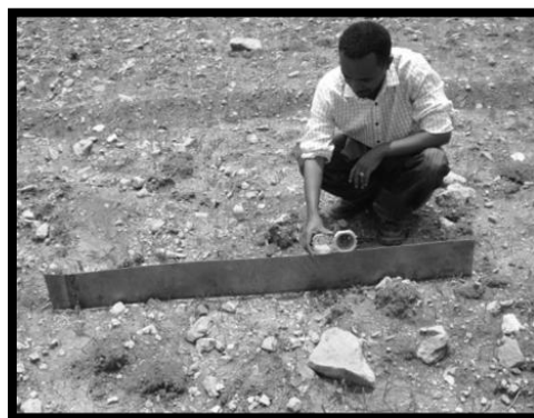
Figure 3.11 Slope measurement on flat object to smooth out the micro-relief
