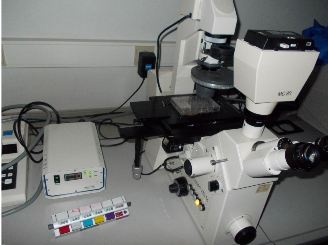
Figure 9. Counting viable and non-viable cells with an inverted fluorescence microscope (Axiovert 135M with a 20x objective; Carl Zeiss, Jena, Germany).
