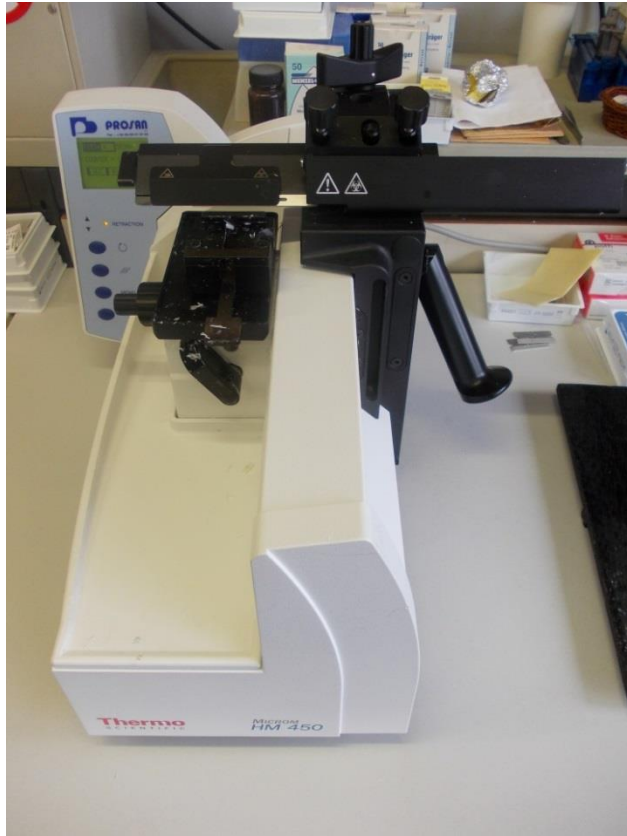
Figure 11. Microm HM 450 sliding microtome by Thermo Scientific (Waltham, Massachusetts, USA).
