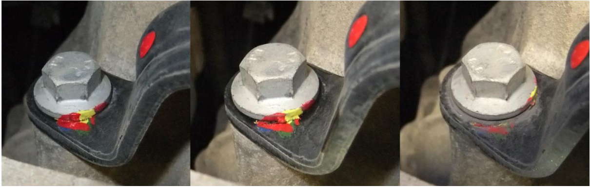
Appendix Figure B 26: From left to right: bolt 4 torqued at 8,6Nm, after 25 passages, after 40 passages
