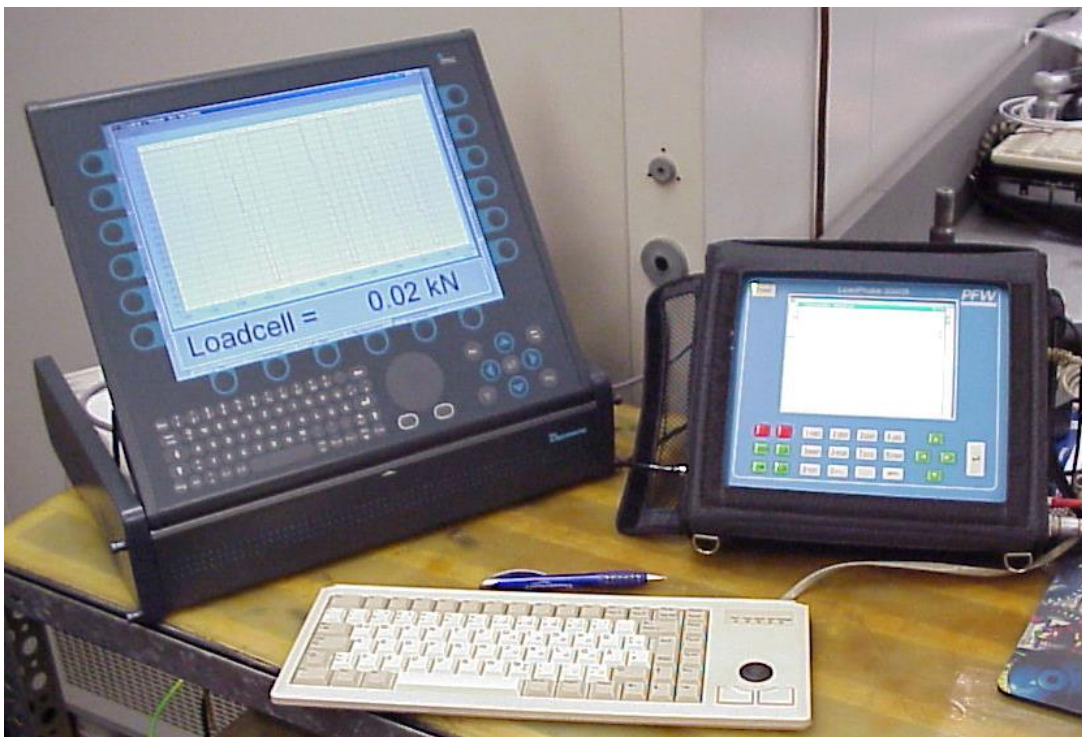
Appendix Figure B 19: On the left the load cell readout for calibration, on the right the LP3000
