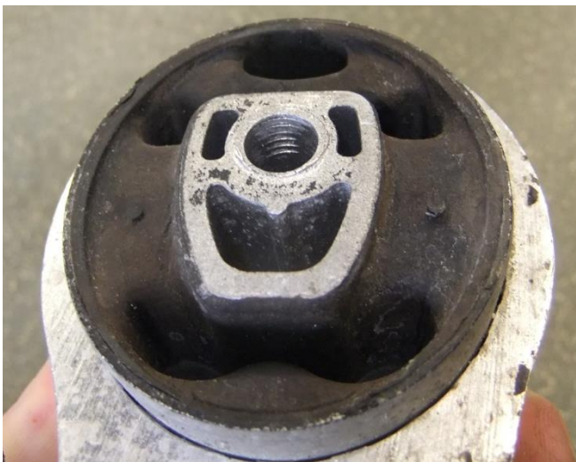
Appendix Figure B 22: Bush on the subframe side of the roll restrictor
