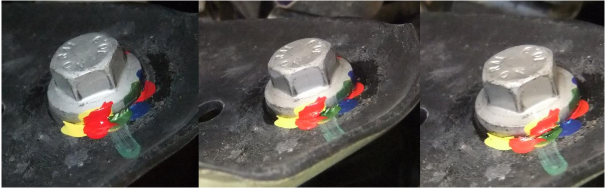
Appendix Figure B 23: From left to right: bolt 1 torqued at 15,2Nm, after 25 passages, after 40 passages
