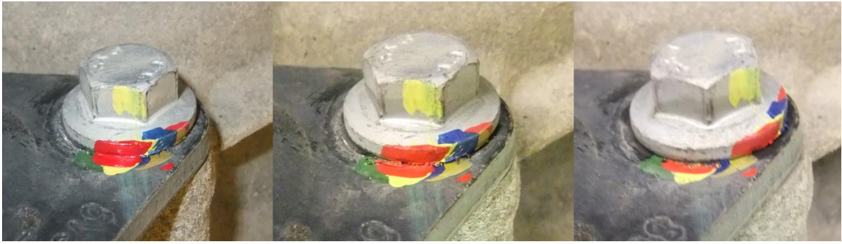
Appendix Figure B 25: From left to right: bolt 3 torqued at 8,2Nm, after 25 passages, after 40 passages
