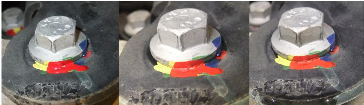
Appendix Figure B 24: From left to right: bolt 2 torqued at 7,6Nm, after 25 passages, after 40 passages
