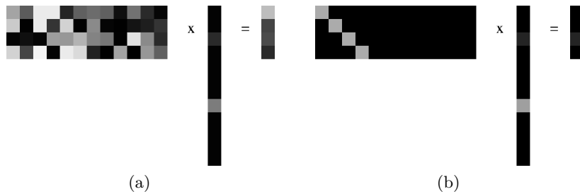
Figure 1.3: Measuring a sparse coefficient vector using (a) an incoherent and (b) a coherent sensing matrix and dictionary combination.
