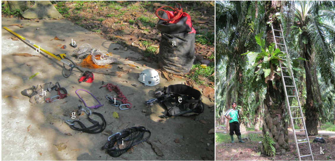
Figure 6.1. On the left climbing equipment ((a) semistatic climbing rope (100m) in orlieb waterproof backpack, (b) nylon lines, (c) pilot ropes, (d) a bigshot, (e) arborist harness, (f) helmet, (g) grigri and sling, (h) hand ascender with foot strop and small pulley, (i) slings, (j) extra rope and several karabiners) and on the right (k) and aluminum ladder
