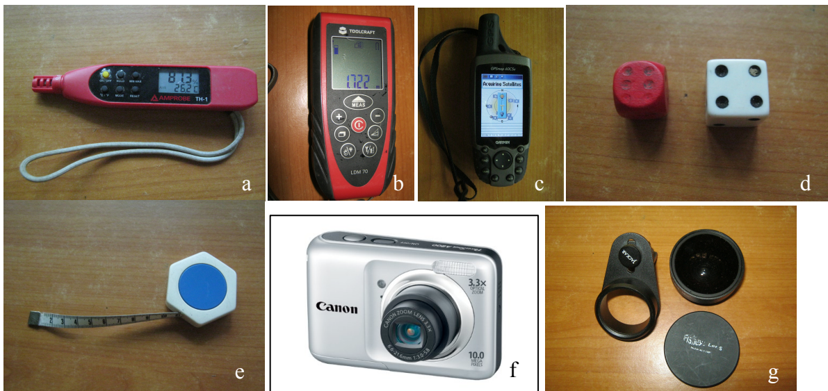
Figure 6.2. Tools for all the necessary measurements: (a) multimeter (Amprobe TH1), (b) range finder (toolcraft LDM 70), (c) gps (Garmin GPSmap 60CSx), (d) dies, (e) measuring tape, (f) compact camera (canon powershot A800) and (g) fish-eye lens (Jackar)
