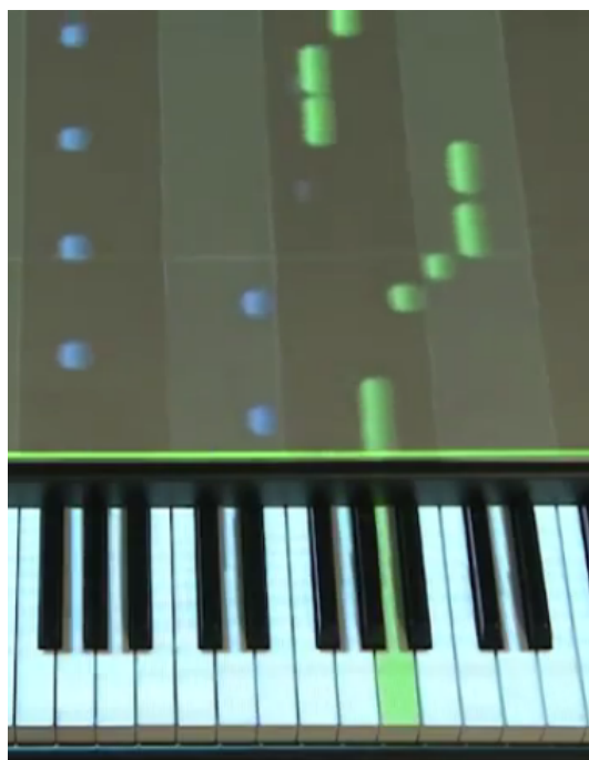
Figure 3.9: Length of note bars signify note duration. Here, note names are disabled on both note bars and piano keys. Keys that are meant to be played are highlighted in the colour of the note bar.
