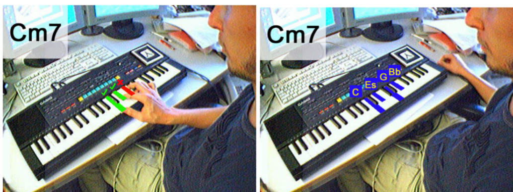
Figure 2.5: The augmented view of the piano keyboard in the Augmented Piano Tutor.
