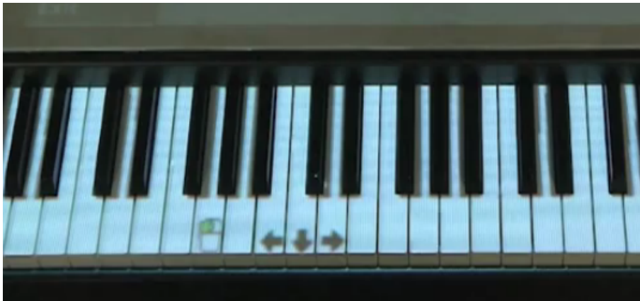
Figure 3.13: The arrow keys mimicked on a piano. The mouse click takes the role of the enter key on the keyboard. Also note that the UP arrow key is not visible on the black key, which is discussed in Section 4.2: Limitations .
