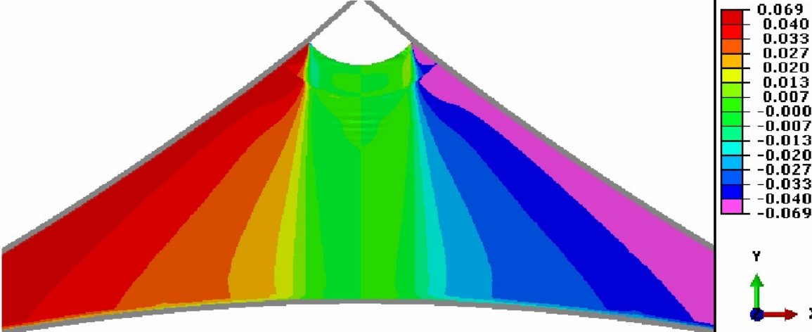
Fig. 107 Vertical strain \epsilon_{22} [-] for model with inversed fiber direction in all membrane parts at top load of L_3 = 7 kN
