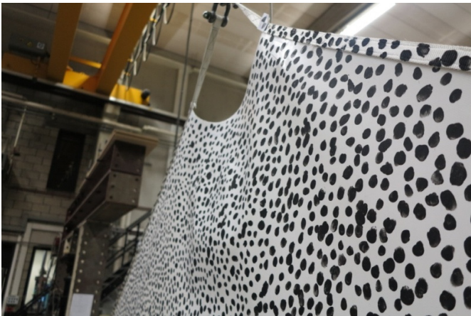
Fig. 37 The slack in the central area after the first load cycle
