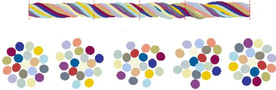
Fig. 1. Results for the twisting of a bundle of 19 initially straight fibres. It shows that outer fibres constantly migrate towards the center, leading to an entangled yarn. Notice, for example, the light blue fibre initially at the outer surface migrates towards the centre and back to the surface.
