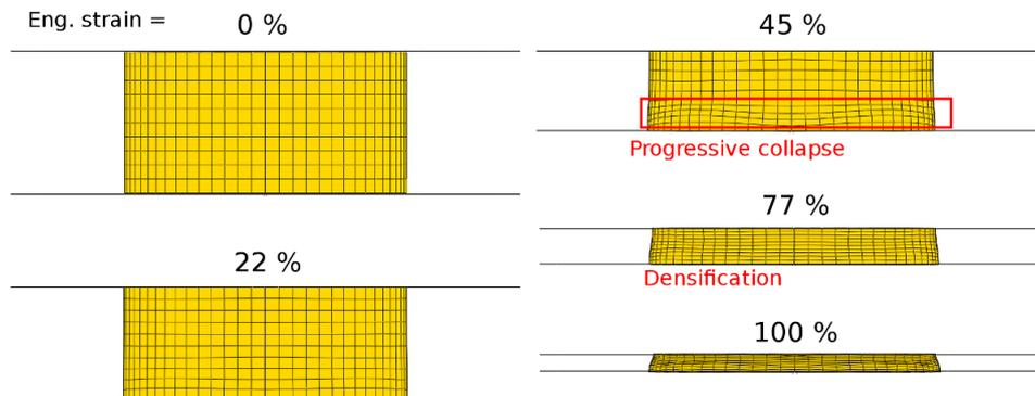
**Figure 6.7:** Compression of a foam disk at different engineering strains showing the progressive collapse of cells in the material.
