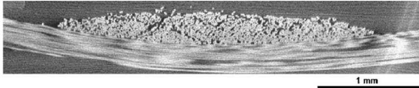
**Figure 3.11:** Experimental observation of the fibres in a yarn.[30]
