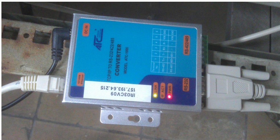
Figure F.1: Standard connection of Multor 610 to DAQ
