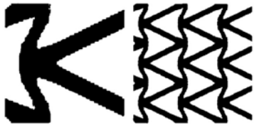
Fig. 7. Image of microstructures with negative Poisson ratio. Courtesy of [3].
