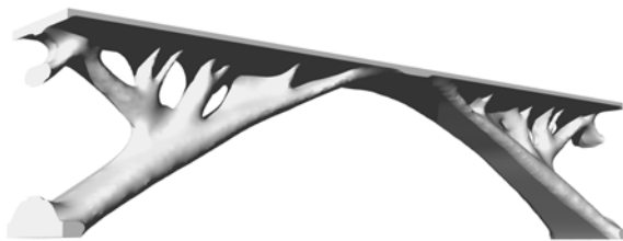
Fig. 4. Perspective view on an optimized 3D design domain. Model extracted from Abaqus and rendered in Rhinoceros.
