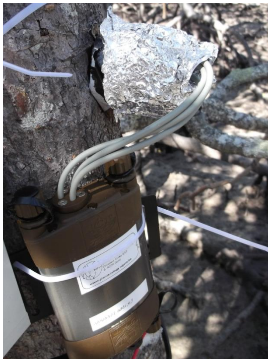
Figure 2.7 Picture of an installed HRM sensor. The needles are shielded from radiation with some insulation and reflective aluminum foil to prevent temperature gradients influencing the sap flow measurements.
