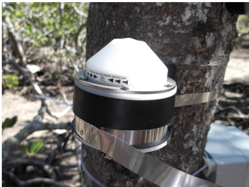
Figure 2.5 A band dendrometer attached to a R. stylosa with dendrometer tape.
