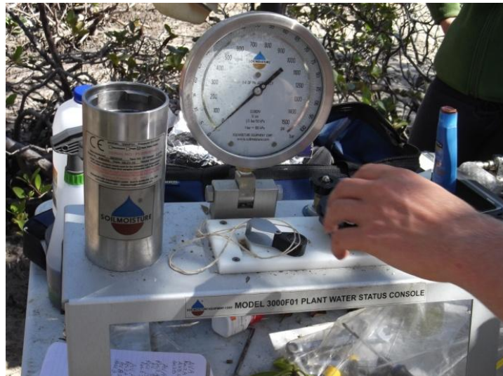
Figure 2.11 The pressure bomb has a pressure chamber in which the leaf or branch is exposed to elevated pressures. A lead cover is used to make the chamber airtight. The pressure gauge is used to read hydrostatic sap pressures. By using magnifying glasses, a higher accuracy and consistency can be achieved.
