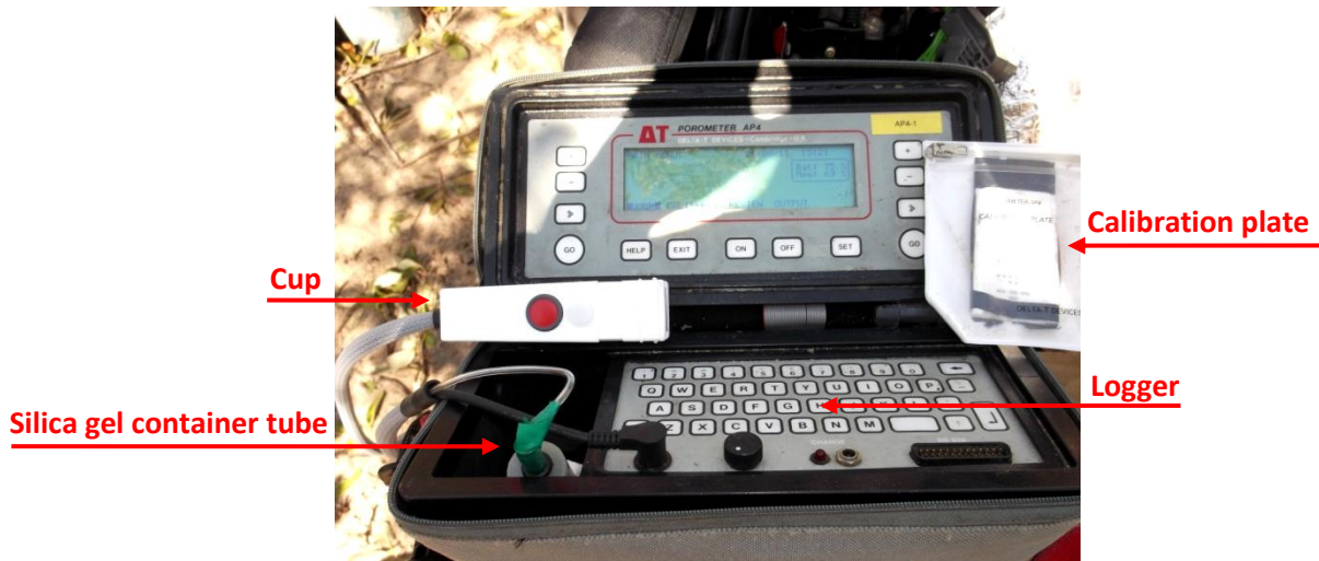
Figure 2.10 The porometer consists of a logger, a cup which needs to be clamped on a leaf to measure stomatal resistance and a calibration plate in a pouch. The end of the tube enters a container tube, filled with silica gel used for drying the air.
