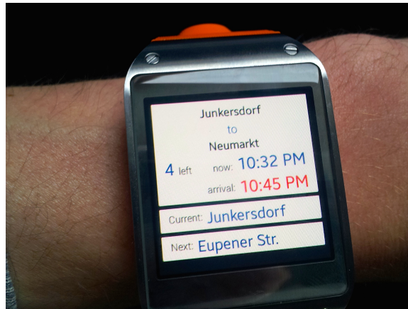
Figure 4-3: Screenshot of the SubwayPS smartwatch application that provides basic feedback to the user without needing to take the smartphone out of their pocket.
