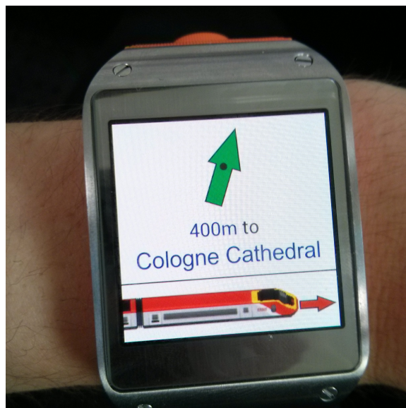
Figure 4-4: Screenshot of the SubwayPS smartwatch application that provides guidance on in which direction to exit the final station to reach a certain POI.
