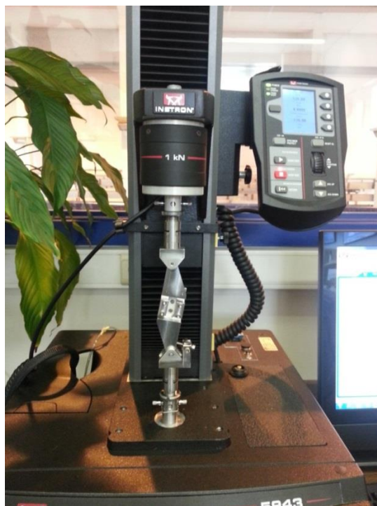
Figuur 23. Two-rail shear testopstelling.
