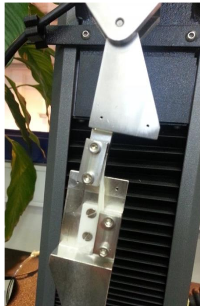
Figuur 26. Verlengde testlengte two-rail shear test.
