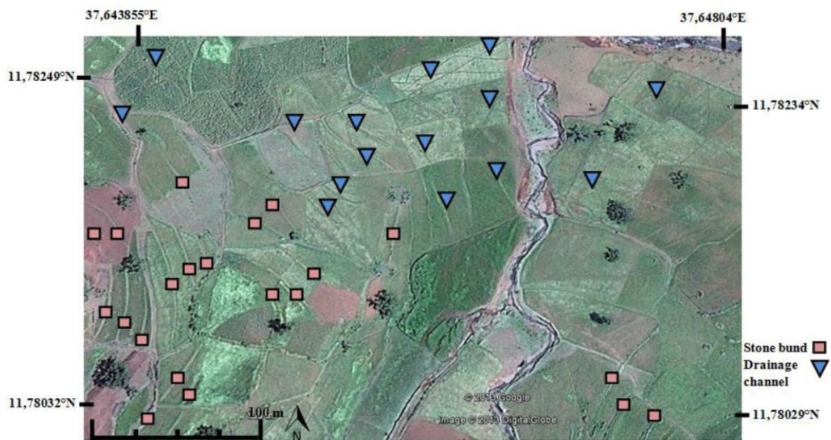
Figure 8. Google Earth image showing drainage ditches and stone bunds. Source: Own editing of Google Earth image.
