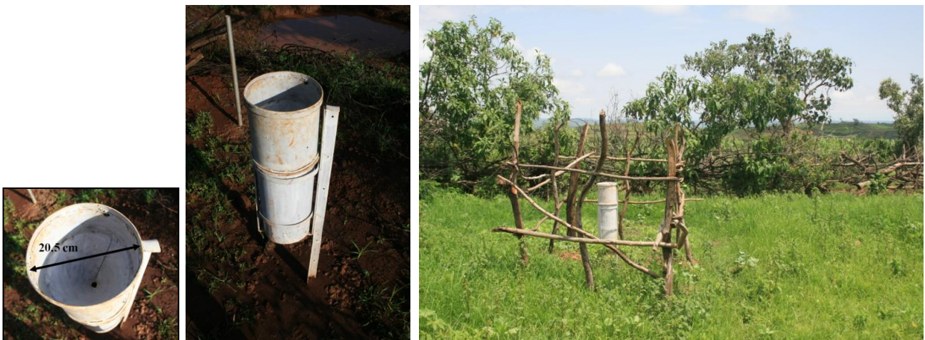
Figure 12. Rain gauges installed in Wanzaye (Ethiopia) after the NMSA rain gauges, with a diameter of 20.5 cm (2013).
