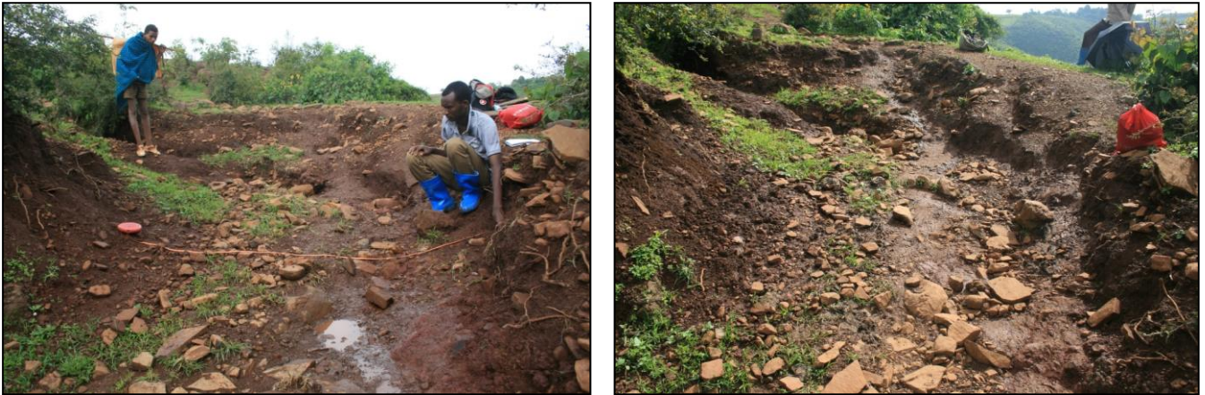
Figure 13. Example of the photographs of the outlet channel for subcatchment 1 on which the collective group evaluation for the parameters defined by Cowan (1956) for Manning's roughness coefficient are based (Wanzaye, Ethiopia, 2013).
